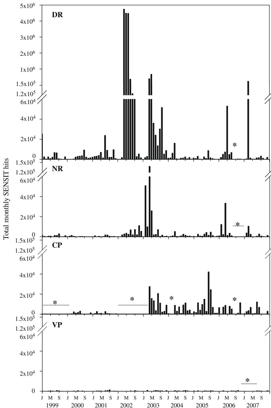
**Fig. 5.** Total SENSIT impacts per month at the four sites. An \* alone indicates missing data for one month; an \* with a line indicates missing data for multiple months. Note the broken axis required for the months with large numbers of SENSIT impacts.
