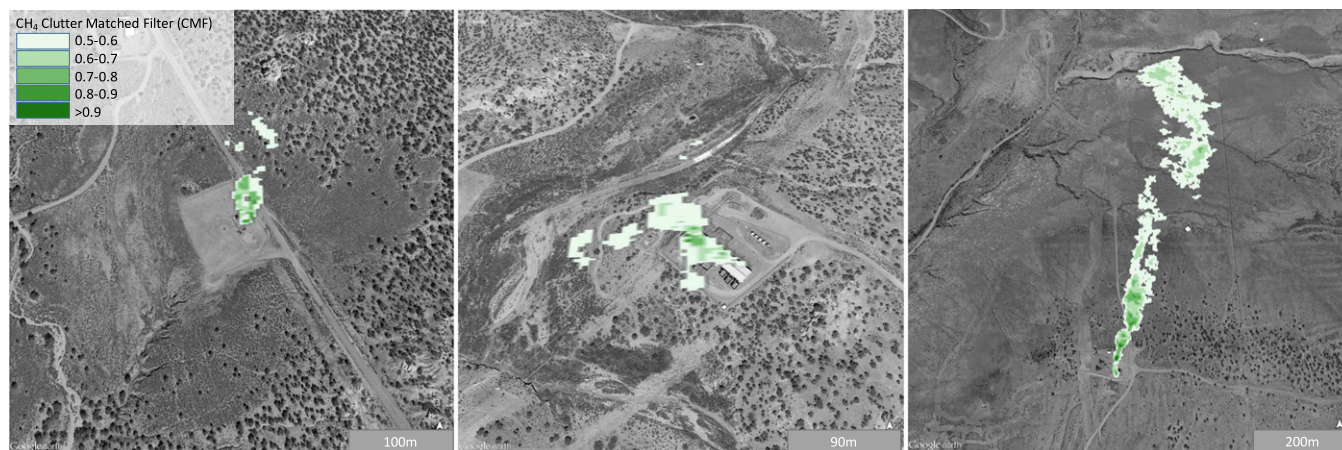
Fig. 2. HyTES methane plume examples for a small, intermediate, and large plume (left to right), related to well pads as well as a storage tank, positively identified by the ground crew ( Movie S1 ). Note the scale difference of the pictures.
